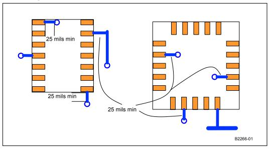
Figure 23 and Figure 24 show good and poor design practices for via placement on surface-mount boards.
